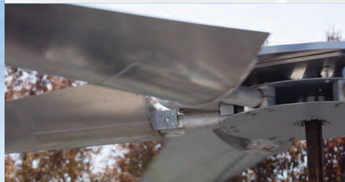
5052 marine grade aluminum blade
