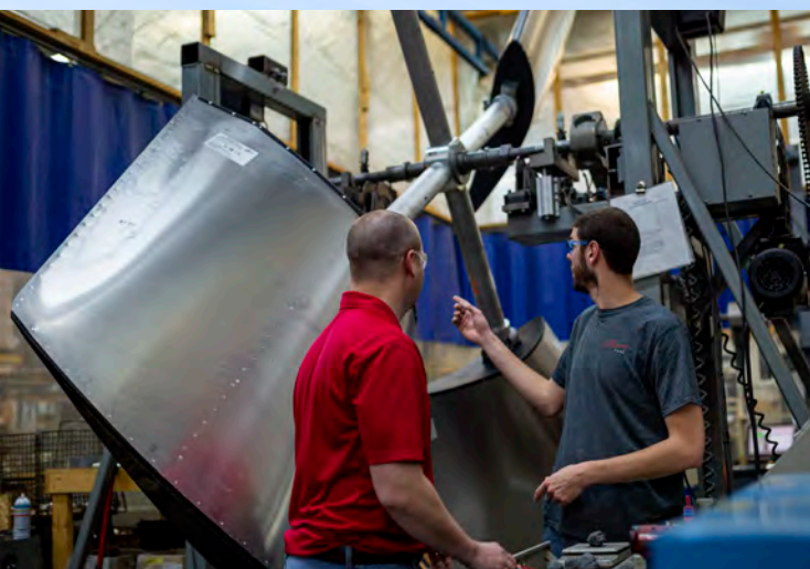
MAG fan being balanced for precision performance
